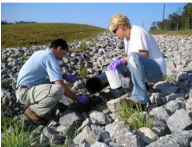
Water Sample Collection from Drainage Pipe
