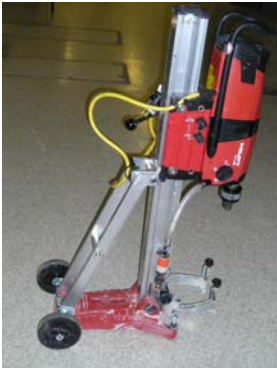
Hilti™ Hammer Drill Used for Concrete Slab Sampling for Soil Vapor Gas
