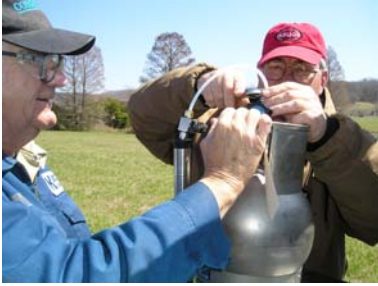
Soil Gas Summa Canister
