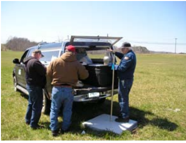
Piezometer Setup for Soil Gas Sampling
