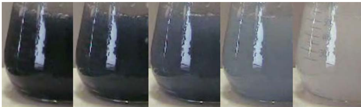
Figure 1. Color change is readily apparent here as solvated solution (sodium dissolved in anhydrous ammonia) is converted to caustic in seconds with titration by water.
